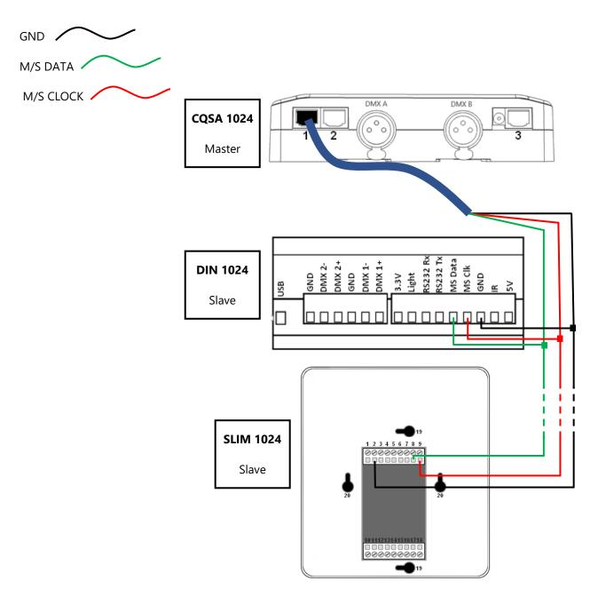
USER MANUAL – How to configure a Master-Slave installation
