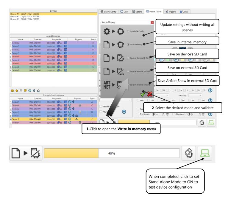
With Stand-Alone mode ON, it's possible to check that all interfaces are correctly configured. After turning on this mode, wait 5 seconds while not using the software. Once the device screens display "00", you can now press the master device buttons to confirm that the same buttons are simultaneously activated on all slave devices.
